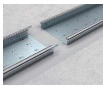
**Laying trunking bases**The trunking bases are routed along the intended course and the side profiles added. Connecting pieces are inserted at the joints.
