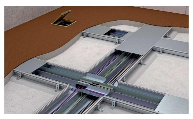
The open, screed-flush OKA-T trunking system is used for cable routing and the installation of electrical resources in the underfloor area. The floor trough and trunking cover are made from galvanised sheet steel with a zinc coating of 275 g/m² according to EN 10327 DX51D+Z275-N-A-C.
