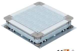
Underfloor junction and branch box for screed-covered underfloor installation ducts with sheet steel side walls. To mount installation units in the mounting lid (to be ordered separately). Height can be infinitely adjusted to the nominal screed height (rapid adjustment possible) and the screed can be worked flushed to the screed scraping edge. With noise decoupling option after screed laying and can be used with system accessories, also for heavy-duty application.
