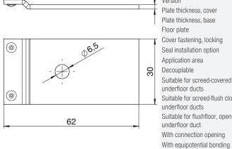
Mounting opening cover N Other Version Plate thickness, cover 1,50 mm 1,00 mm Plate thickness, base Floor plate Cover fastening, locking Seal installation option Application area Screed-covered Decouplable Suitable for screed-covered  $\checkmark$ underfloor ducts Suitable for screed-flush closed underfloor ducts Suitable for flushfloor, open underfloor duct With connection opening
